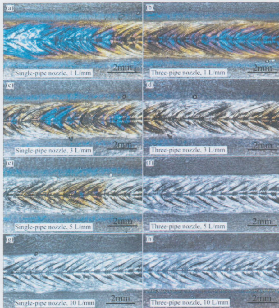
Fig. 5 Influences of gas nozzle type and gas flow rates on surface appearance of welded seams
